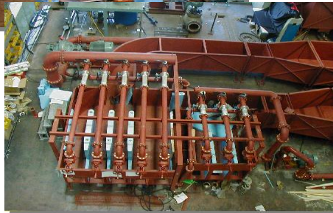
Sump Model Study for MACAO COLOANE-B CCPP Intake
