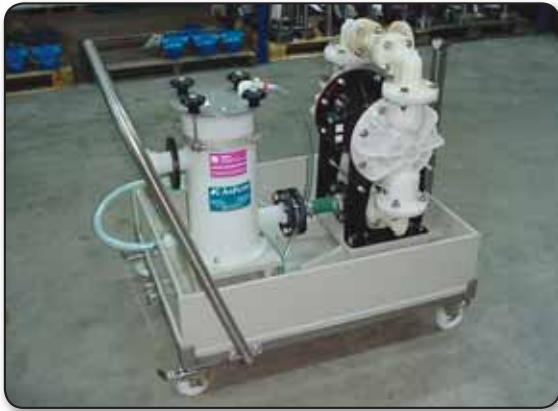
Distributor fabricated portable filtration cart with standard duty non-metallic pump.
