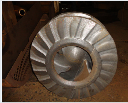
F6145WRT1A05 Impeller 2,088 hours inspection
