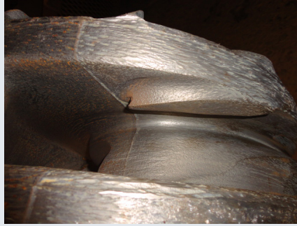
F6145WRT1A05 Impeller 2,088 hours inspection
